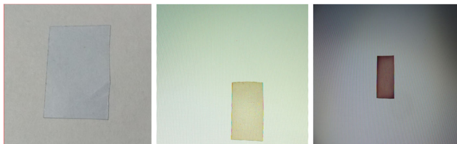
Fig. 2 Change in color of films sorbed with I_3^- and after treatment with variamine blue dye
