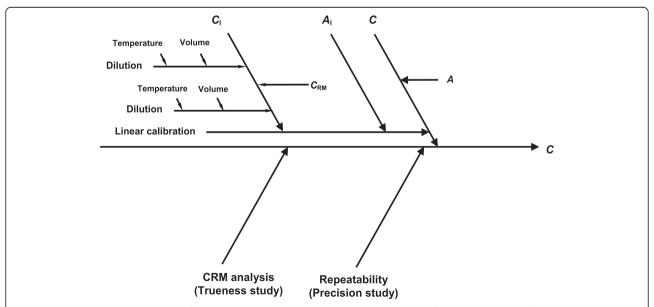
**Figure 1 Cause and effects diagram of uncertainties.** The uncertainties in the measurement of mass concentration of elements in aqueous herbal extracts are obtained using ICP-OES.
