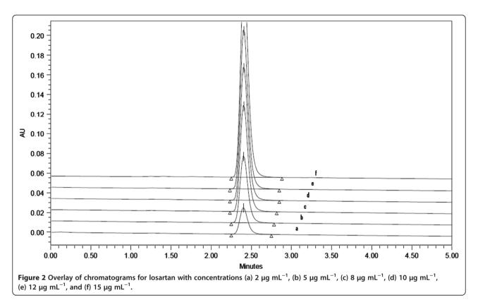
These were obtained by a series of dilutions of the LOS stock solution. Precision study was performed at the LOQ level also. LOQ solution was injected six times (n = 6) and the %RSD values for the obtained peak area and retention time were calculated.
