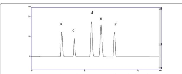
Figure 2 Representative chromatograms showing peaks of (a) cetirizine, (c) tiaprofenac acid, (d) flurbiprofen, (e) ibuprofen, and (f) mefenamic acid.
