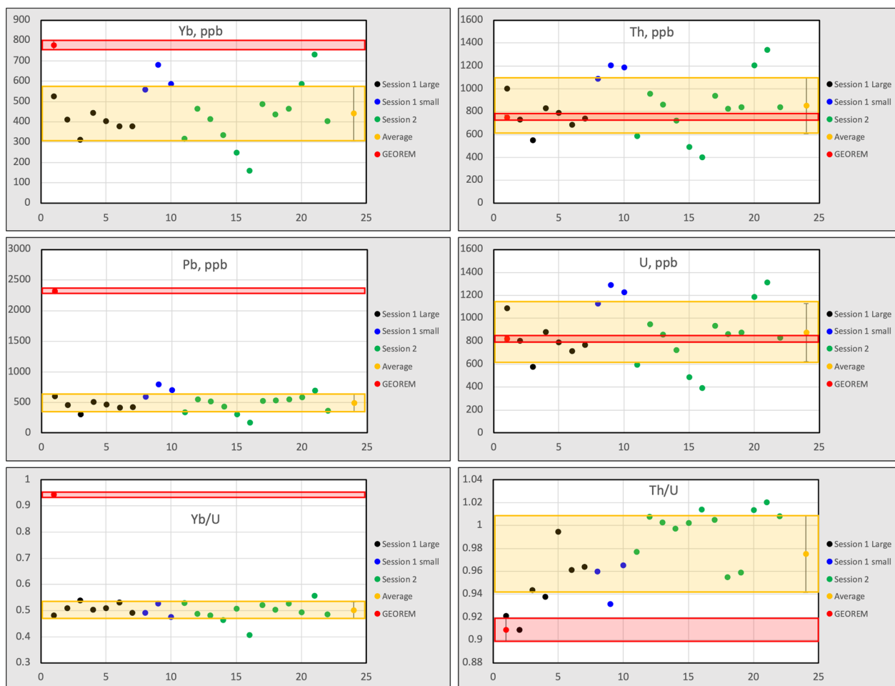
Fig. 3 Concentrations of Yb, Th, U and total Pb, and Yb/U and Th/U ratios, in NIST SRM 615 glass. The Pb concentrations are sums of concentrations of individually measured Pb isotopes. Session 1 “large” spot analyses—black symbols, session 1 “small” spot analyses—blue symbols, session 2 analyses—green symbols. The average values with SD uncertainties are shown with yellow symbols and shaded areas. The accepted values with uncertainties (Jochum et al. 2016) are shown with red symbols and shaded areas
